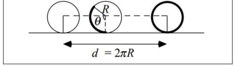
When the object makes one complete revolution, the object has moved a distance equal to the circumference, and each point on the exterior has touched the ground once.
