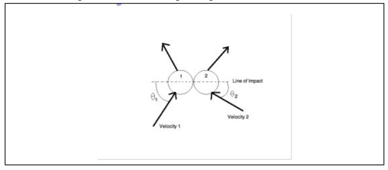
III) Line of impact: The instant when two bodies just collide, the line joining their centres is called the line of impact.
